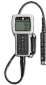
Fig. 5: YSI multiprobe sensor (temperature, salinity, oxygen)
